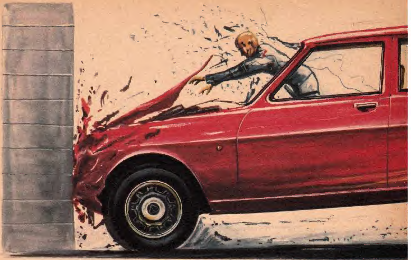
A car being tested for safety by staging a mock crash and using a dummy in the place of the driver. A typical car-testing dummy, showing the photographic markings on the head, face and other injury areas.
